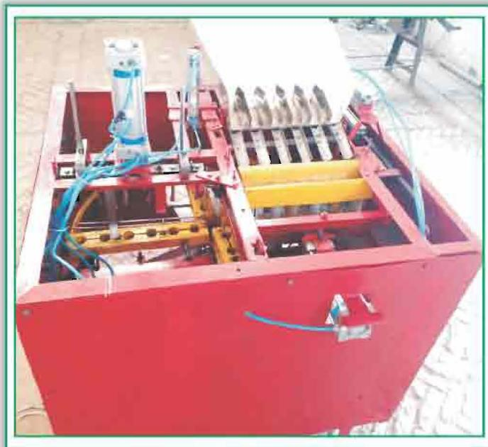
Fig 1- Pneumatic assisted coring device
